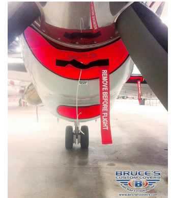
ENGINE PLUGS PREVENT BIRD NEST FOD. Piper Saratoga Engine Cowling Bird's Nest Engine and Oil Cooler Inlet Plugs
