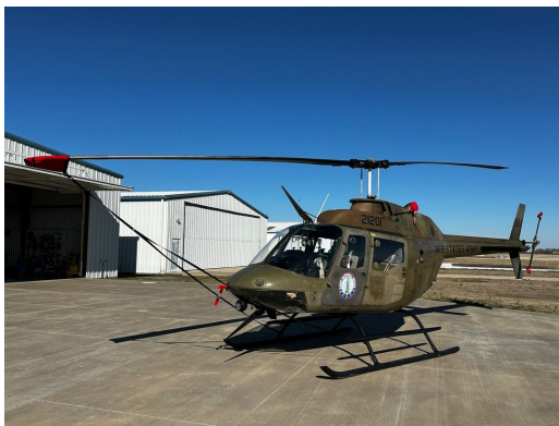
Bell 206B JetRanger Blade Tie, Tail Rotor Tie, Pitot Cover, Exhaust Cover
