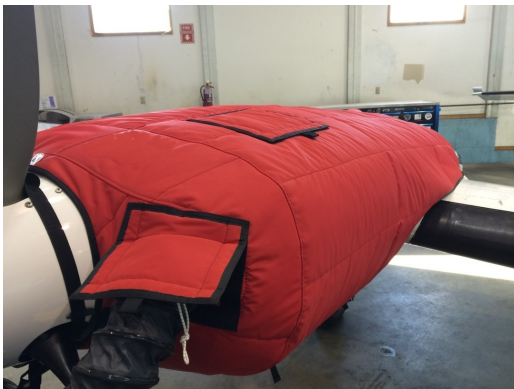
Cessna 402 Insulated Engine Cover with Heater
