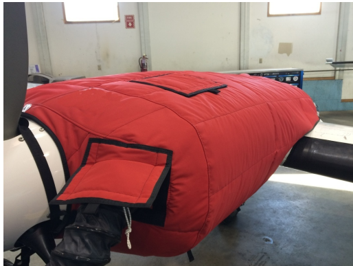
Cessna 402 Insulated Engine Cover with Heater
