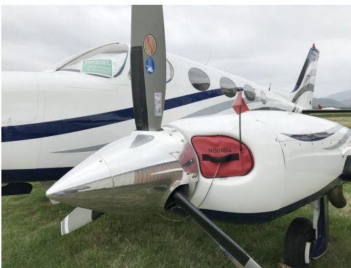
Cessna 340 Engine Inlet Plugs
