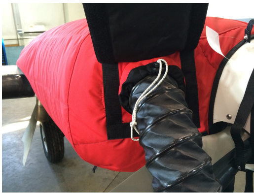
Cessna 402 Insulated Engine Cover with Heater
