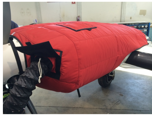
Cessna 402 Insulated Engine Cover with Heater
