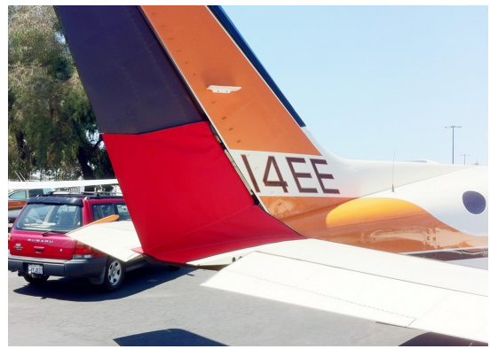
Cessna 414 Rudder Openings Cover (bird barrier)
