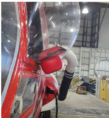
Boeing Vertol CH-47 Logger Window Plug
