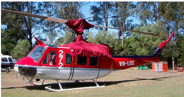
Bell 204/205 Engine/Mid-Cabin Cover, Main & Tail Rotor Covers
