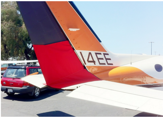
Cessna 414 Rudder Openings Cover (bird barrier)
