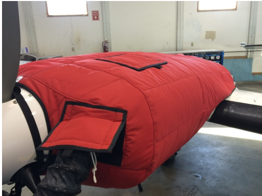
Cessna 402 Insulated Engine Cover with Heater
