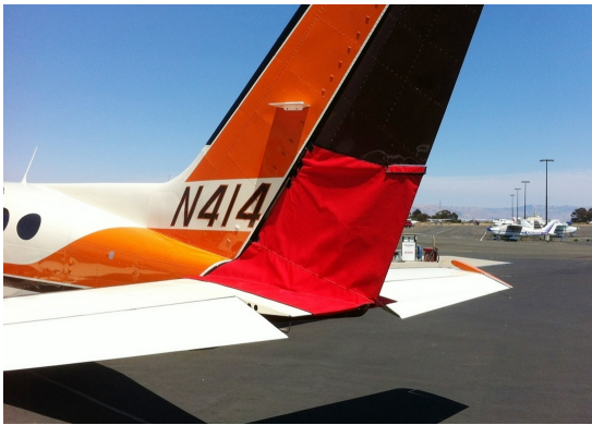
Cessna 414 Rudder Openings Cover (bird barrier)
