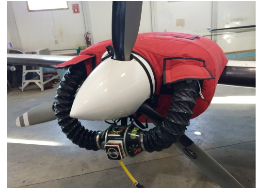
Cessna 402 Insulated Engine Cover with Heater
