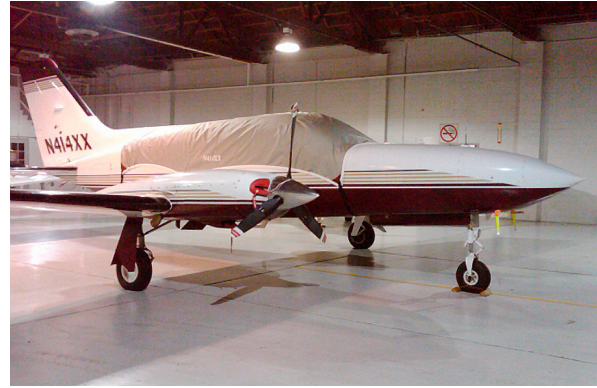
Cessna 414 Canopy Cover and Engine Inlet Plugs
