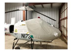
Enstrom 280FX Bubble, Main Rotor Mast, Tail Rotor Covers on Enstrom F280FX Enstrom F28A, F28C Bubble Cover "Flat Nose"
