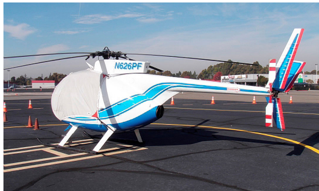
MD500C Bubble Cover with Wire Strike detail
