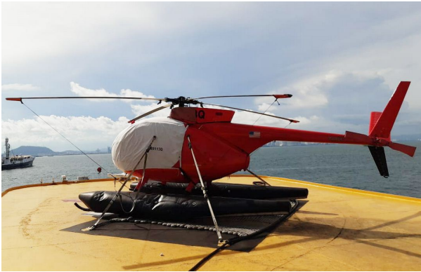
Hughes 500C (369HS) Bubble Cover, Blade Tie-Downs
