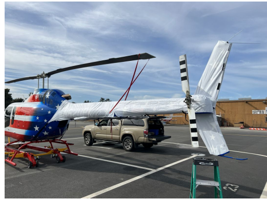
Bell 505 Tailboom & Stabilizer Covers, test fit cover
