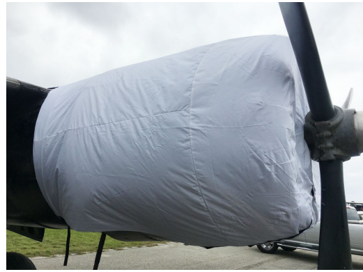
Douglas A-26 Engine Cover, test fit cover
