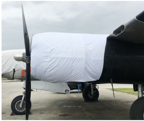
Douglas A-26 Engine Cover, test fit cover
