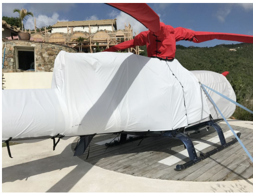
Aerospatiale Gazelle AS341 Bubble, Rotor Mast, Blade, Engine & Tailboom Covers (some are test fit covers)
