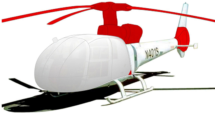
Gazelle Bubble, Abbr. Engine, Rotor Hub, Blades & Fenestron Covers (Illustration)
