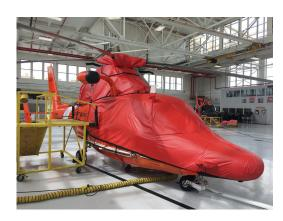
Aerospatiale AS365N2 Bubble, w/Extended Nose/Radome U.S. Coast Guard HH-65 Dolphin Bubble, Engine & Rotor Mast Covers
