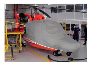
U.S. Coast Guard HH-65 Dolphin Bubble, Engine & Rotor MH-65C Bubble Cover, extended Nose/Radome Model, padded over windows, P/N: A365-210
