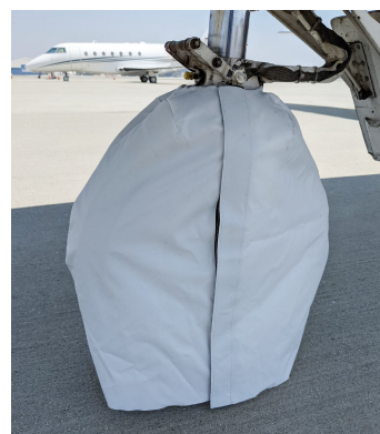
CJ1 Nose Gear Tire Cover, test fit
