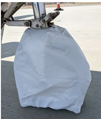
CJ1 Nose Gear Tire Cover, test fit
