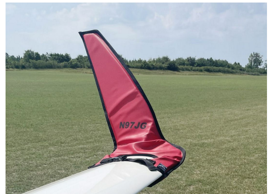
Schempp-Hirth Ventus-2B winglet/wingtip pads
