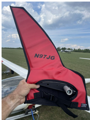
Schempp-Hirth Ventus-2B winglet/wingtip pads
