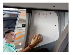
Airbus Helicopter EC130 B4 Side Window Heatshields
