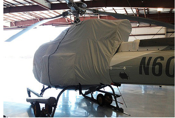
AS350 B3 Main Body Cover (Covers Bubble/Cabin, Engine Area and Exhaust). Squirrel Cheeks.
