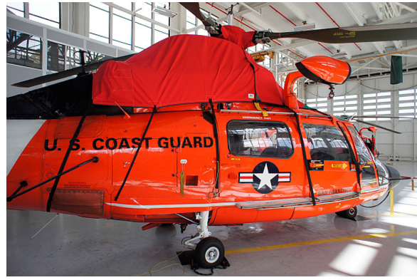
MH-65C Engine Area, Rotor Hub, Swash Plate Aperture Cover set, P/N: A365-210
