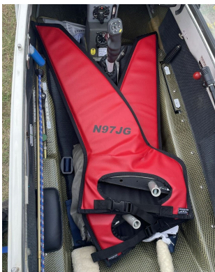
Schempp-Hirth Ventus-2B winglet/wingtip pads
