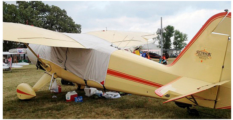
Stinson Reliant Over-the-top Canopy Cover and Engine Cover
