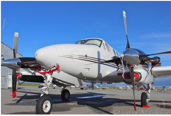
King Air C90A Engine Plugs and Pitot Covers
