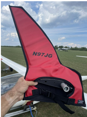
Schempp-Hirth Ventus-2B winglet/wingtip pads
