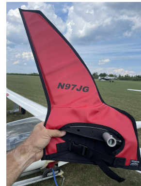
Schempp-Hirth Ventus-2B winglet/wingtip pads
