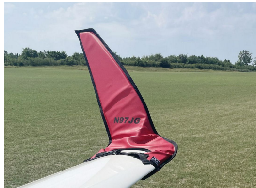
Schempp-Hirth Ventus-2B winglet/wingtip pads
