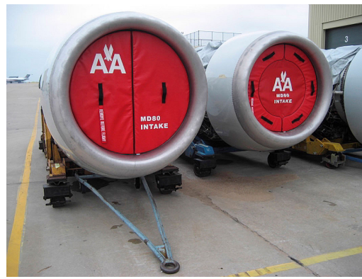
MD-80 JT8D Intake Plugs, Solid Foam folding type & Mesh Center folding type
