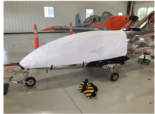
Bede BD-5 Canopy/Nose Cover, test fit cover
