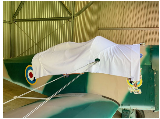
Bowers Flybaby Canopy Cover, test fit design
