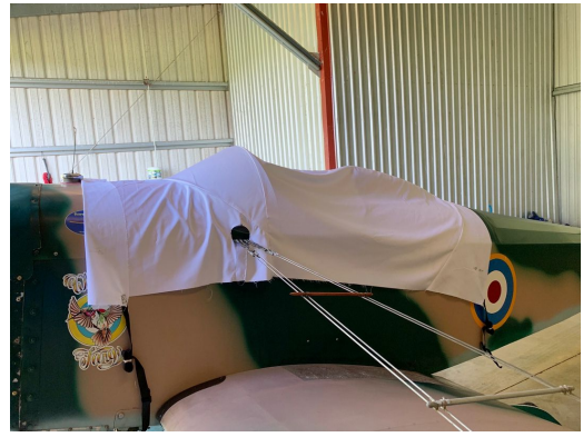
Bowers Flybaby Canopy Cover, test fit design
