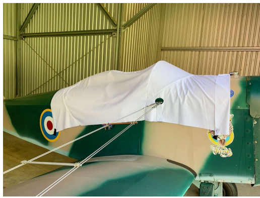
Bowers Flybaby Canopy Cover, test fit design
