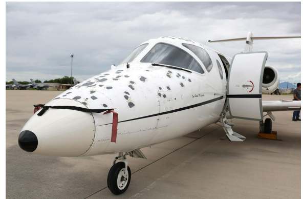
Raytheon Beechjet Hail Damage, and Pitot Covers
