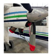
Britten-Norman Islander, prop tie/exh. cover and inlet plug for BN-2T Allison Britten-Norman Islander Engine Inlet Plugs & Prop Engines.
