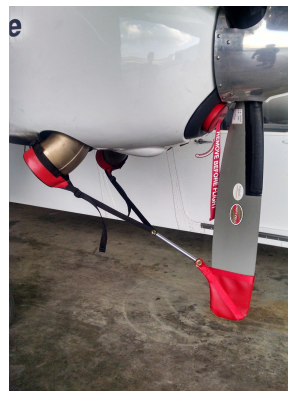
Britten-Norman Islander Engine Plugs Britten-Norman Islander, prop tie/exh. cover and inlet plug for BN-2T Allison Engines.
