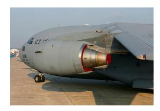
C-17 Bypass and Exhaust Plugs (illustration)
