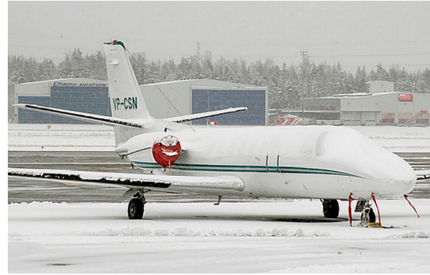
Cessna 560 Engine Inlet/Exhaust Covers, Pitot Cover Set
