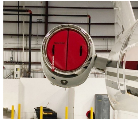
Embraer Legacy 500 Engine Inlet Plugs, folding type
