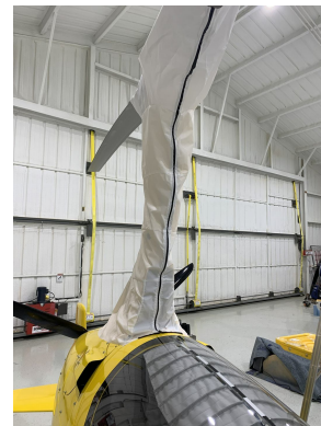
Calidus Gyrocopter Rotor Mast Cover, test fit cover
