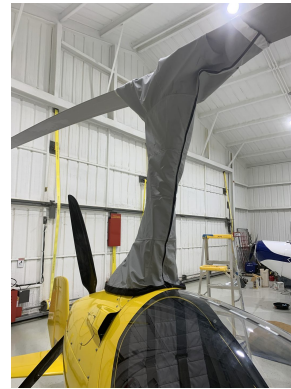
Autogyro Calidus Gyrocopter Rotor Hub/Mast Cover
