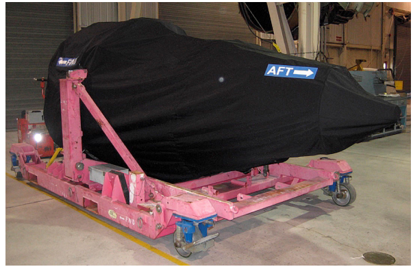
CFM-56-7 Off-link Engine Shipper/Transport cover, w/ Exhaust Cone, fully enclosed
