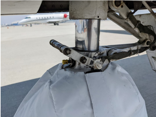
CJ1 Nose Gear Tire Cover, test fit
