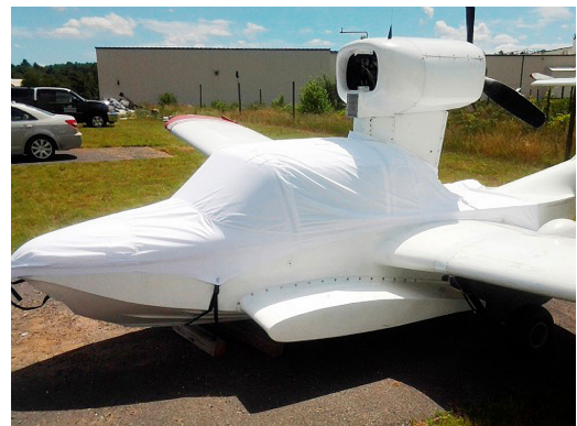
Taylor Coot Canopy/Nose Cover, test fit cover
