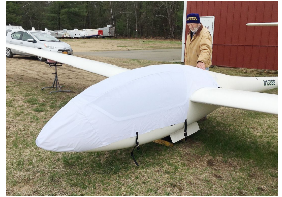
Grob 102 Astir CS Canopy/Nose Cover (test fit)
