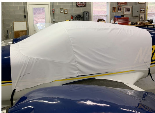
Wing Derringer Canopy Cover, test fit
