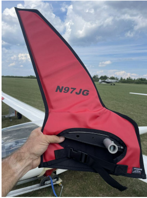
Schempp-Hirth Ventus-2B winglet/wingtip pads
