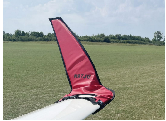
Schempp-Hirth Ventus-2B winglet/wingtip pads
