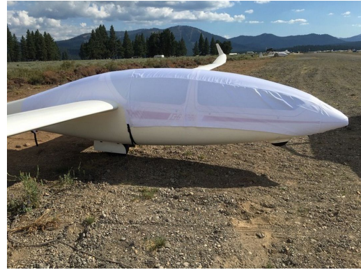
DGF 1000 Canopy/Nose with Turtledeck Extension (test fit cover)
