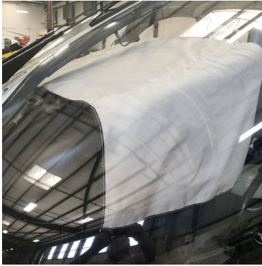
Eurocopter EC-135 Instrument Panel Heatshield Cover
