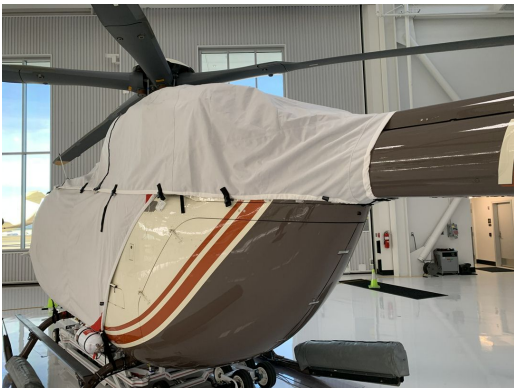
Eurocopter 145 Engine Area Cover, Bubble Cover
