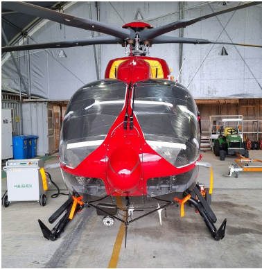
Airbus Helicopter H145D3 Windshield Heatshields, Engine Plugs
