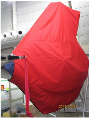
Airbus EC145 Tailfan Housing Fenestron Cover
