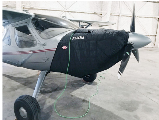
Glasair Aviation Glastar, Sportsman 2+2 Insulated Engine Cover
