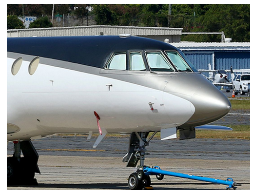
Dassault Falcon 50 Cockpit HeatShields
