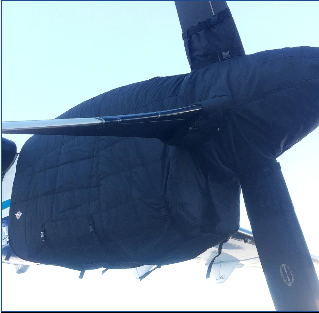
ATR-72-202 Insulated Engine & Prop Hub Covers
