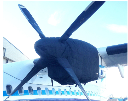
ATR-72-202 Insulated Engine & Prop Hub Covers
