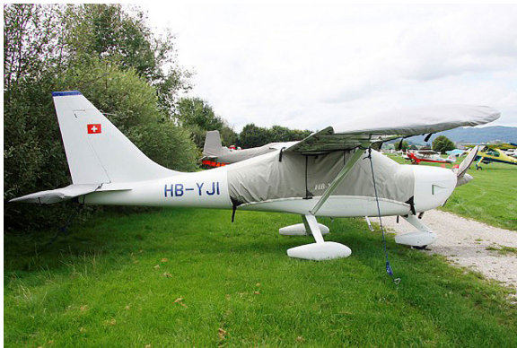
Glastar Canopy, Wings, Horizontal Stab. & Prop Covers
