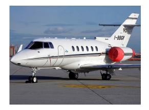
Hawker 900XP Tri-Fold Engine Intake/Exhaust Cover Set
