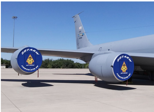
BOEING KC-135 Tambourine Type Double Fold Intake Covers, Custom Mesh Insert & IUID's with custom Imprint
