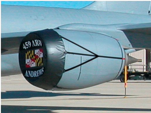
KC-135 "soft" type Intake Cover
