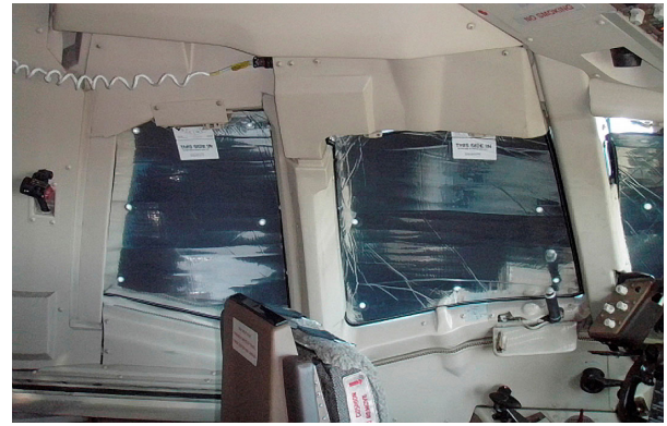
Boeing 767 Cockpit HeatShield set
