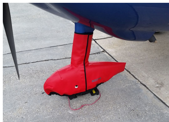
Lancair Columbia Nose Wheelpant/Strut Cover
