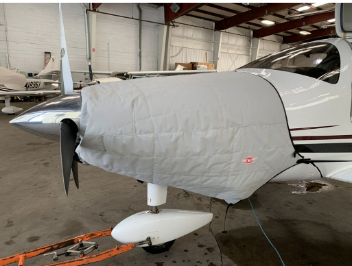
Cessna Corvallis Insulated Engine Cover
