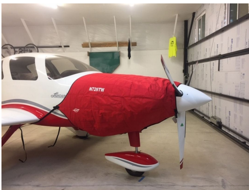
Lancair ES Insulated Engine Cover, Fully Enclosed
