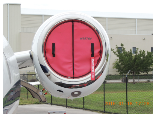
Embraer Legacy 500 Engine Inlet Plug, folding type
