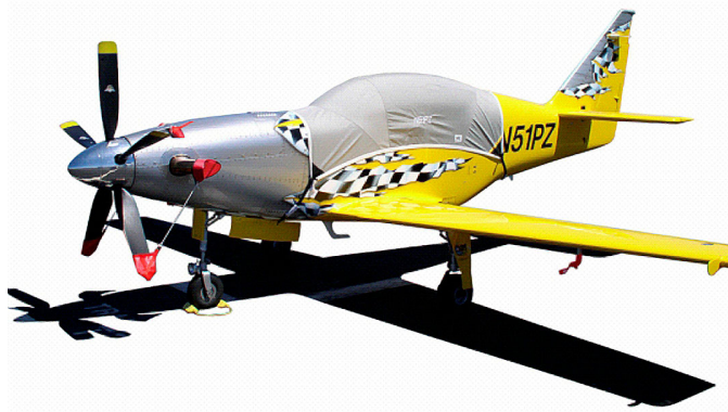
Legend Canopy Cover, Prop Ties, Exhaust Covers & Intake Plugs
