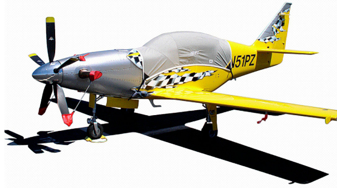
Legend Canopy Cover, Prop Ties, Exhaust Covers & Intake Plugs
